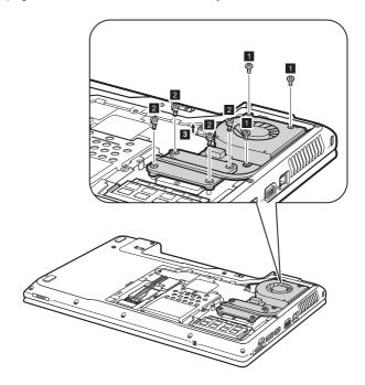
When installing: Make sure that the fan connector is attached firmly to the system board.
